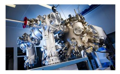
The Compact 21 system will enable the laboratory, already equipped with RIBER machines, to enhance its versatility by adding a new ultra-high vacuum (UHV) chamber to its existing lines, and to multiply its processes or share its equipment with other research groups.
